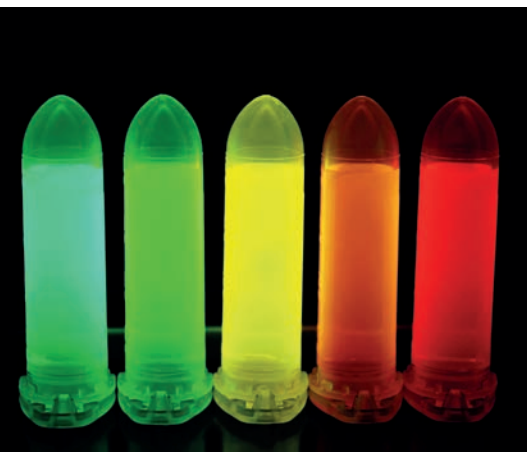
The color of quantum dots generally changes with their size (as shown here), but microporous silica can be used to produce nanometer-scale quantum dots whose color also varies with temperature.
