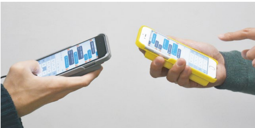
Figure 2: Smartphone-based haptic text-based chat system with audio-vibrotactile feedback for sense of presence. © Kazuki Sakurada, SFC TOUCH LAB
